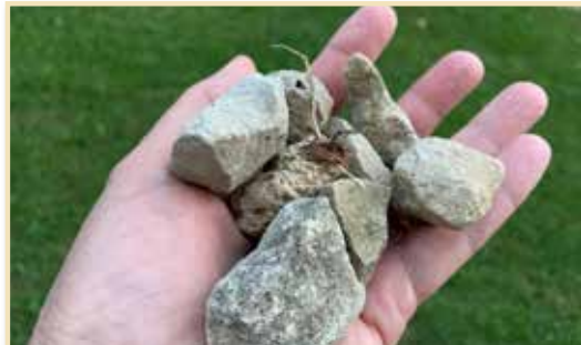
Two to five-inch rock provides scour protection at inlets and outlets.
