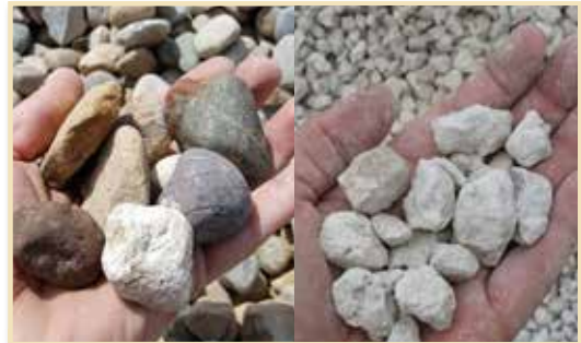
1-inch washed field rock and crushed limestone rock.
