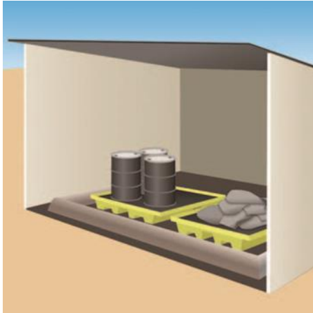
Shelter used to protect materials from rain. Secondary containment used to capture any spills.
