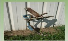
Slotting or ripping tool used for subsurface soils on treatment side.
